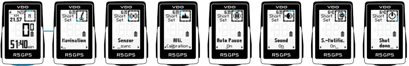
You can access the quick menu when the training has started or is in AutoPause. In the quick menu you only have access to the most important training functions and settings. While exercising, press and hold the START button to open the quick menu.
