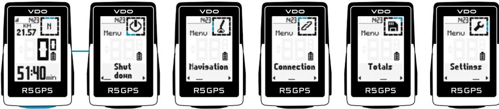
You can reach the main menu if the training has not yet started or is in a stopped state (ATTENTION not AUTOPAUSE). Via the main menu you can access all available settings as well as a smartphone or external sensors for the first time.
